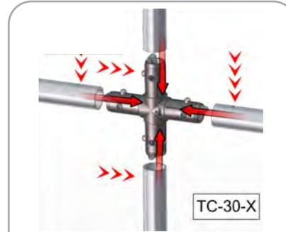
Using TC-30-X junction to connect frame in the middle.
