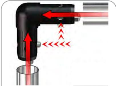
Assemble frame corners using TC-30-90. Label codes will be on backside of tube. It is best to assemble frame laying flat.
