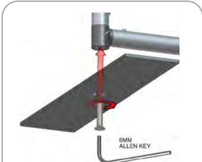
Using provided allen key, secure feet to bottom of frame by screwing bolt.
