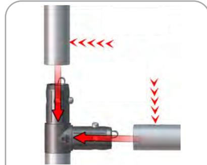
Using TC-30-T junction to connect sides of frame to middle section.
