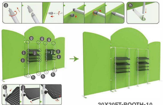
Clip into hanging boards based on directions of three-way clips & tightening with thumb screws, clip F-shaped bar onto hanging board with thumb screws. 20X20FT-BOOTH-10
