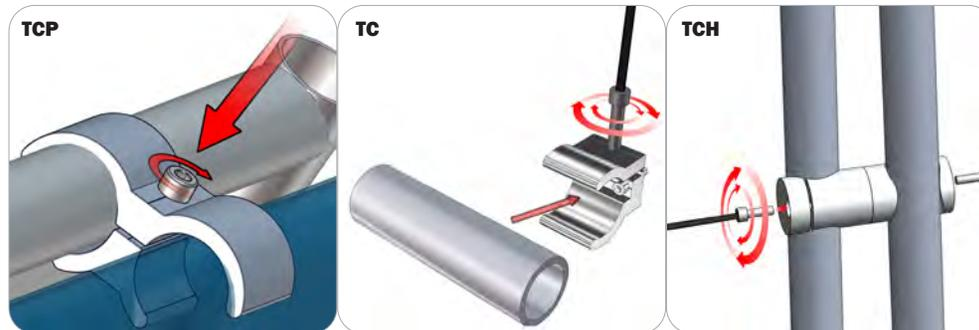
Be sure to fully assemble all frames before using clamps. With the clamp unlocked, place one tube of the first frame into the mouth of the clamp. Place the second tube (if applicable) into the second mouth of the clamp. With both frame's tubes in the clamp, be sure to lock securely, but do not overtighten.
