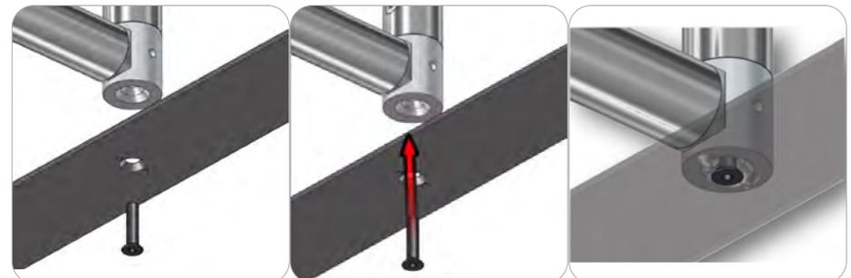
First, loosen the set screw that is on the PLT-BP-LN114, then attach the base plate with the LN114-SCRW insert. Once the base plate is in the desired position, fasten the set screw to hold the insert in place.
