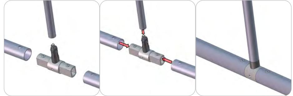
For connections, Compress one unlocked end of the connector and slide it through one tube end. Compress the other end of the connector and slide the second tube on. Next, Slide 30mm tube down onto TC-30-D-ES50-S-ASY (pictured in the "included in your kit" section above), til snap into place.
