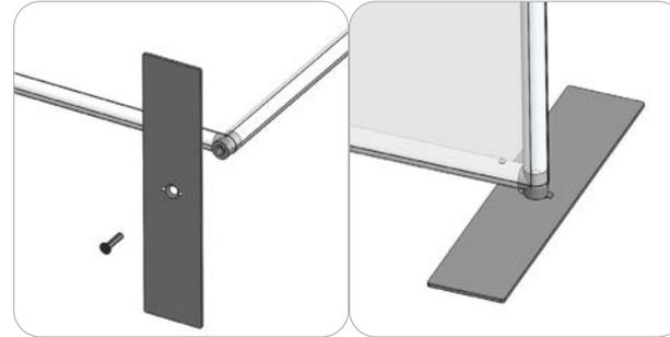
Join the frame to the stabilizing bases. Fasten the screw carefully using your allen key tool. Be sure to fasten securely, but do not overtighten.
