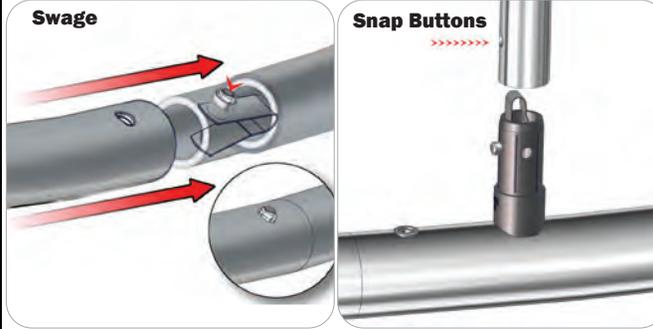
Locate the snap button on the connector or swage tube. Locate the hole on the corresponding tube. Press the snap button with your thumb and slide the tube and connector together so that the snap button snaps fully into the lock hole. To disassemble, press the snap button and pull apart.
